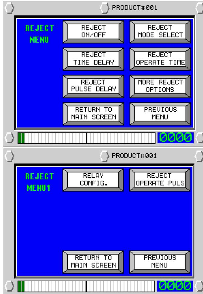
**Reject delay time** - Sets the time between detection of metal and the activation of the reject device. It can be adjusted in tenths of a second from 0-30 seconds.
