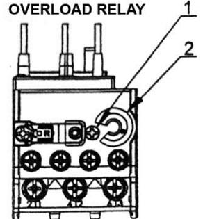
**Warning** - To provide continued protection against fire or shock hazard, the complete overload relay must be replaced if burnout of one or more of the heater elements occurs.
