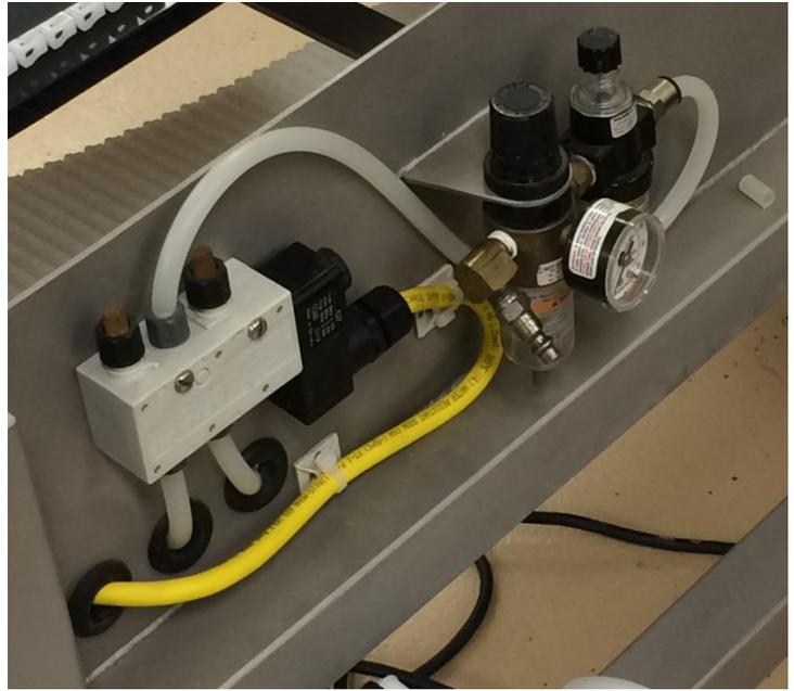
**The yellow button activates the solenoid manually, without tripping the metal detector.**
