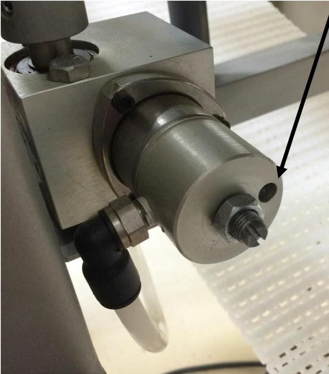
These set screws should only be adjusted with the assistance of the factory.
