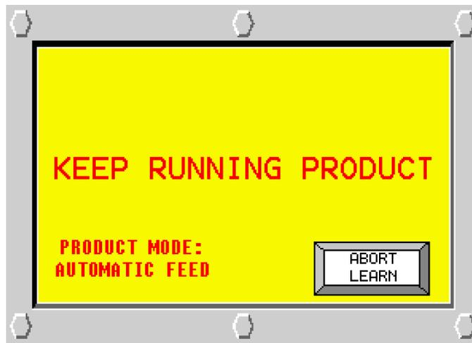
When the “Keep Running Product” screen appears, be sure the conveyor belt is running and allow product to pass through the detector aperture. When the detector has enough samples, the “LEARN SUCCESSFUL” screen will appear.
