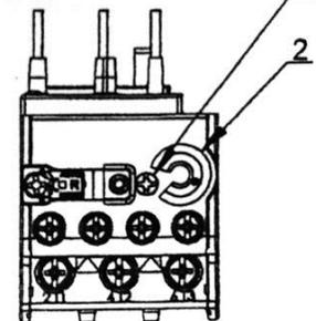
Warning - To provide continued protection against fire or shock hazard, the complete overload relay must be replaced if burnout of one or more of the heater elements occurs.
