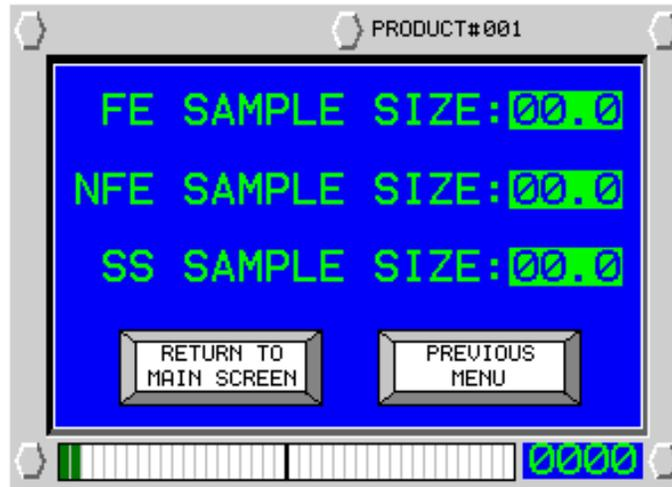
Enter the size of the test wand you will be using during the test. This value will be saved in memory and listed on the data logger along with a time and date stamp upon successful completion of the ferrous test. Enter the desired values for each metal type.
