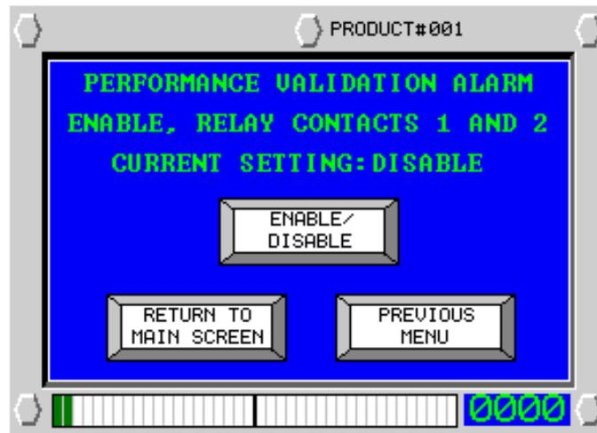
Press the Enable/Disable to enable the relay. The relay will toggle when the performance reminder screen appears and clear when the user selects either Cancel or Begin. An alarm and/or light can be wired to the relay.
