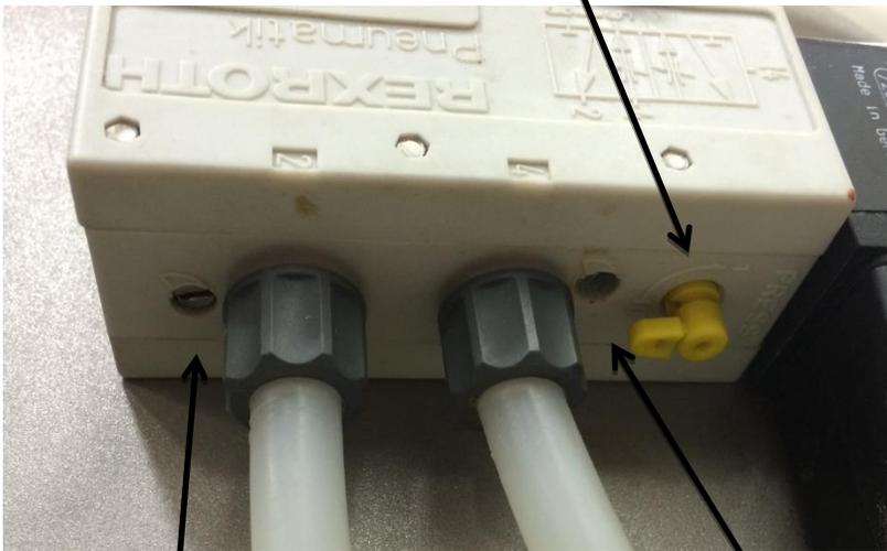
**This set screw controls the retreat rate, or the speed in which the sweep**
